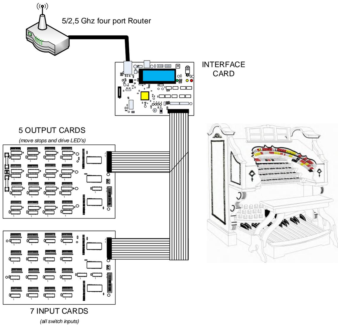
Figure 31 Console Uniflex Setup
