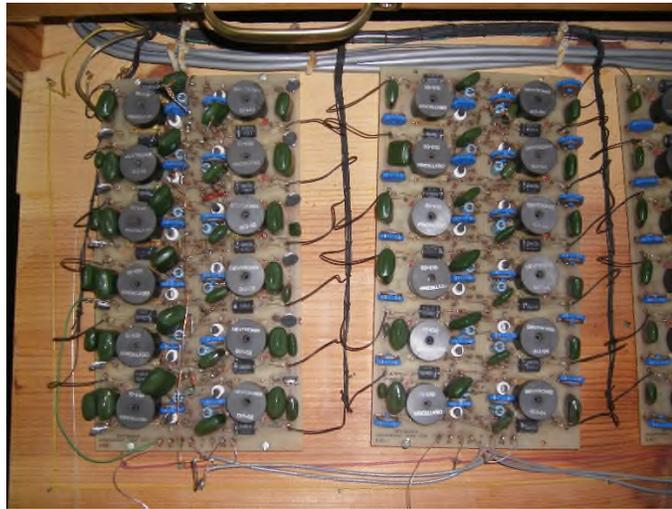
*Figure 9 Oscillator Boards*
