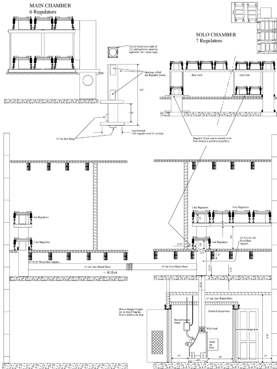
Figure 25 Organ Winding Plan
